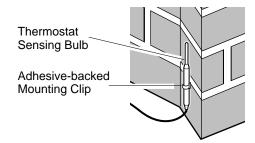
Figure 34 - Locating Thermostat Sensing Bulb on Masonry Fireplace
